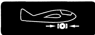
When the airbrake handle is pulled back to its fullest extent, it will also actuate the hydraulic disc brake of the main wheel.
